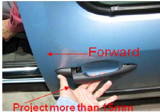
These opening face of these handles do not face either rearwards or downwards so it would seem that they must comply with both Part 1 and Part 2 of section 6.6.2.2.
