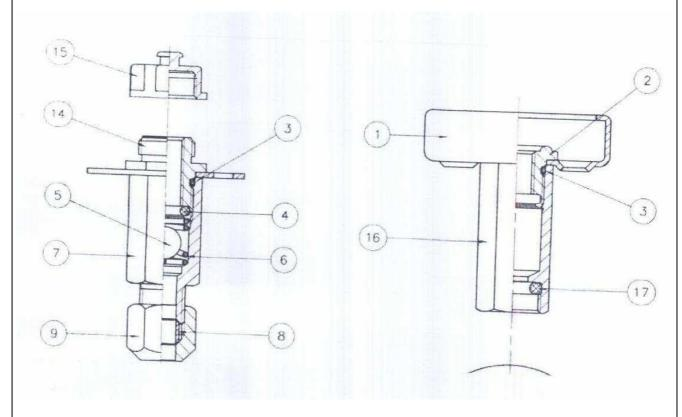
According the above mentioned drawing, this filling unit consists of two parts: the **left** part, with includes the soft-seated non-return valve and is fixed to the vehicle, and the **right** part, which is removable. The two parts are screwed together without any locking security.
