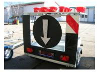
In the case when the trailer is out of intended function and is normally transported on road, there is a problem with "moving traffic signs" or not approved reflective materials or their installation respectively. Pursuant to R 48 (paragraph 2.7.16.) "other retro-reflective plates and signals which must be used to comply with **national requirements** for use as regards certain categories of vehicles or certain methods of operation;" are not considered as retro-reflectors.
