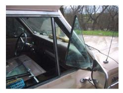
VCA believes that window division bars were excluded from the measurement because they were not significant at the time. But vehicle designs have changed and it is now common to have secondary A pillars – all of the following being approved:
