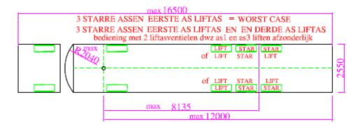
Some manufactures lose business weekly because in other countries a 3 axle configuration with lifting device on the first axle and a wheelbase as drawn is picture 1 here above is allowed. Although this configuration is not compliant to the 1230/2012 Annex 1 Part D 3 manoeuvrability requirements.
