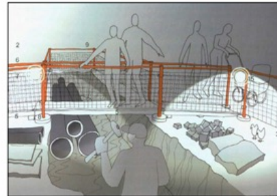
Figures 6 and 7. Examples of arrangements for unobstructed traffic at a worksite.
