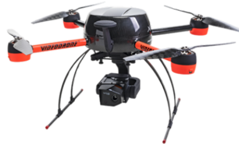
VideoDrone X4L, 6.5kg, 60min endurance
