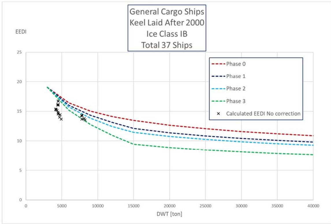
Figure 32: Calculated EEDI for general cargo ships with ice class IB without correction ( $f_i = f_j = 1$ ).
