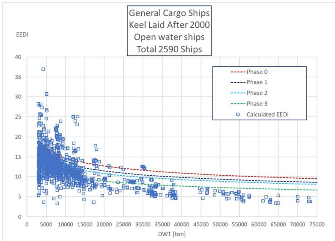
*Figure 29: Calculated EEDI values for the studied open water general cargo ships.*
