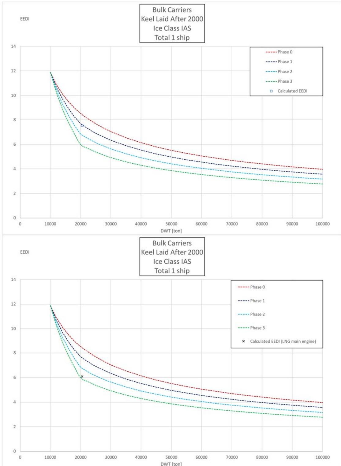
Figure 41: Comparison of calculated EEDI for LNG and MDO as fuel, bulk carriers in ice class IAS.
