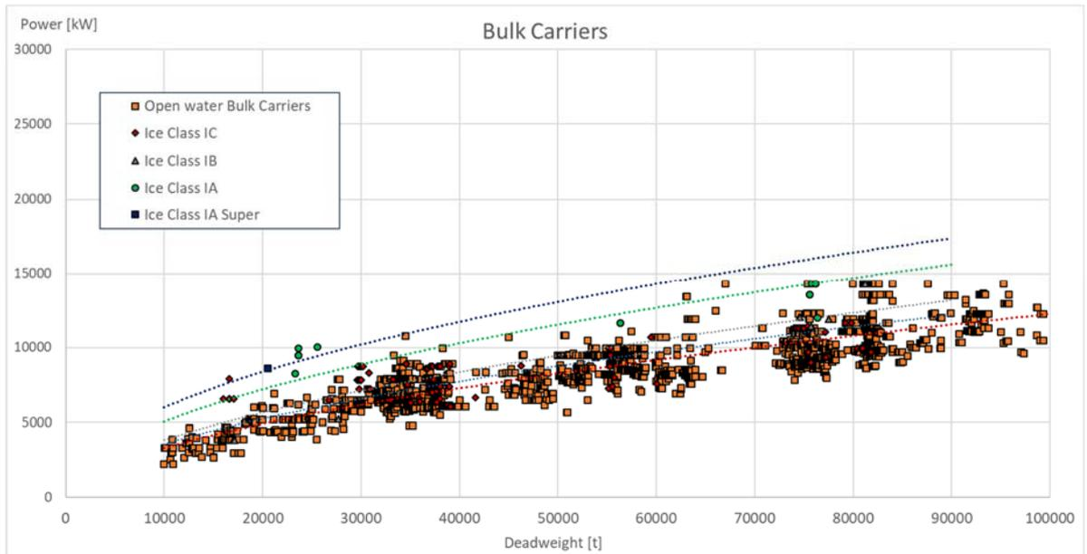
Figure 4: Average engine power of existing bulk carriers with and without an ice class.
