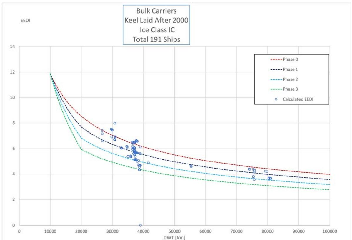
Figure 22: Calculated EEDI for bulk carriers with ice class IC with the proposed new  $f_j$  and  $f_i$ .
