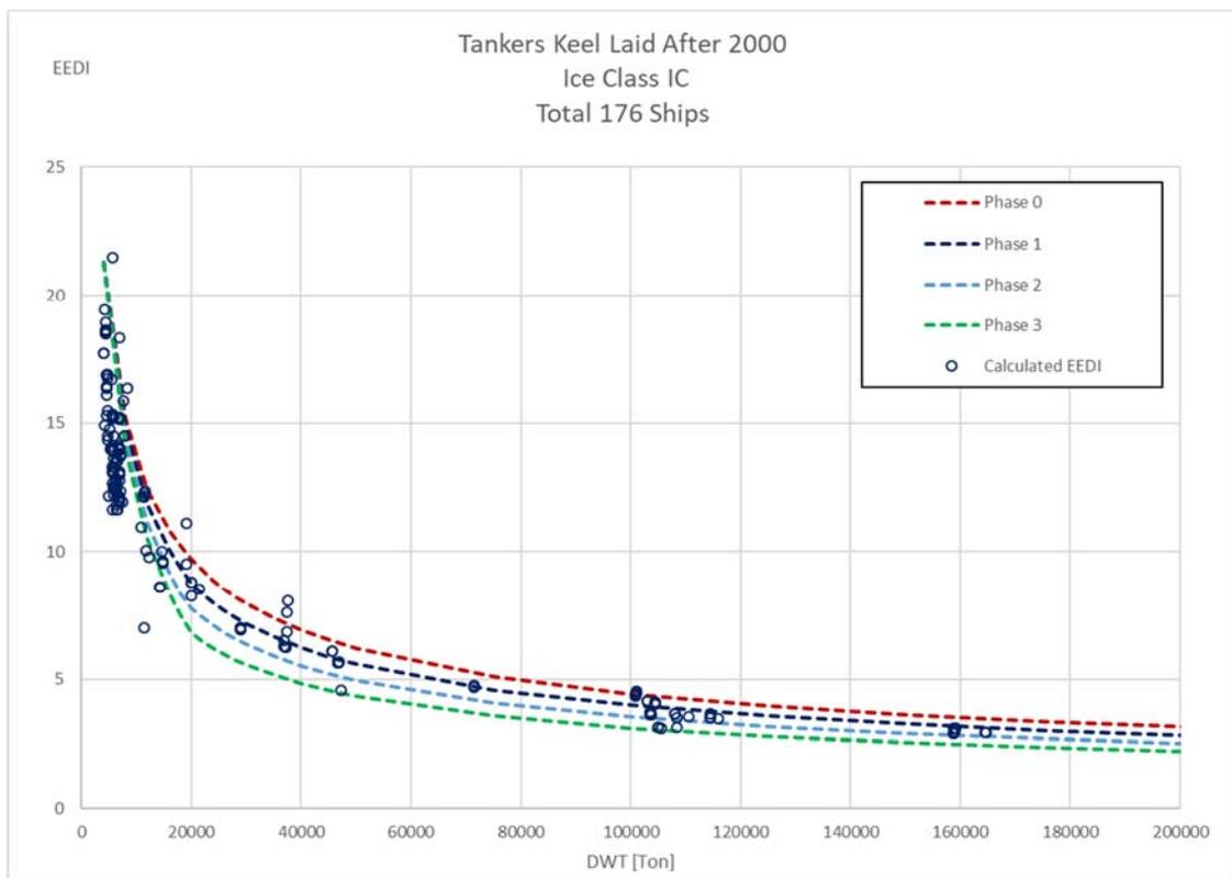
Figure 13: Calculated EEDI for tankers with ice class IC with the proposed new  $f_i$  and  $f_j$ .
