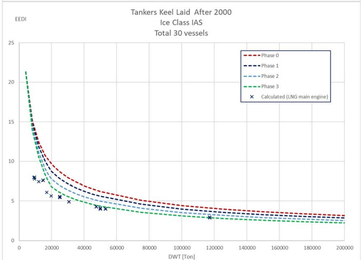
**Figure 39: Comparison of calculated EEDI for MDO and LNG as fuel, tankers in ice class IAS.**
