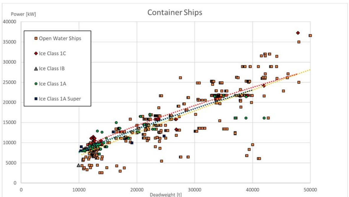
Figure 8. Average engine power of existing container ships with and without an ice class.
