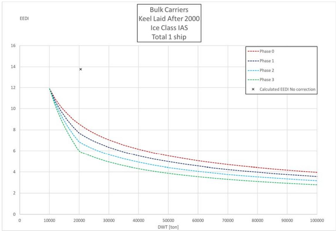
Figure 27: Calculated EEDI for bulk carriers with ice class IAS without correction ( $f_i = f_j = 1$ ).
