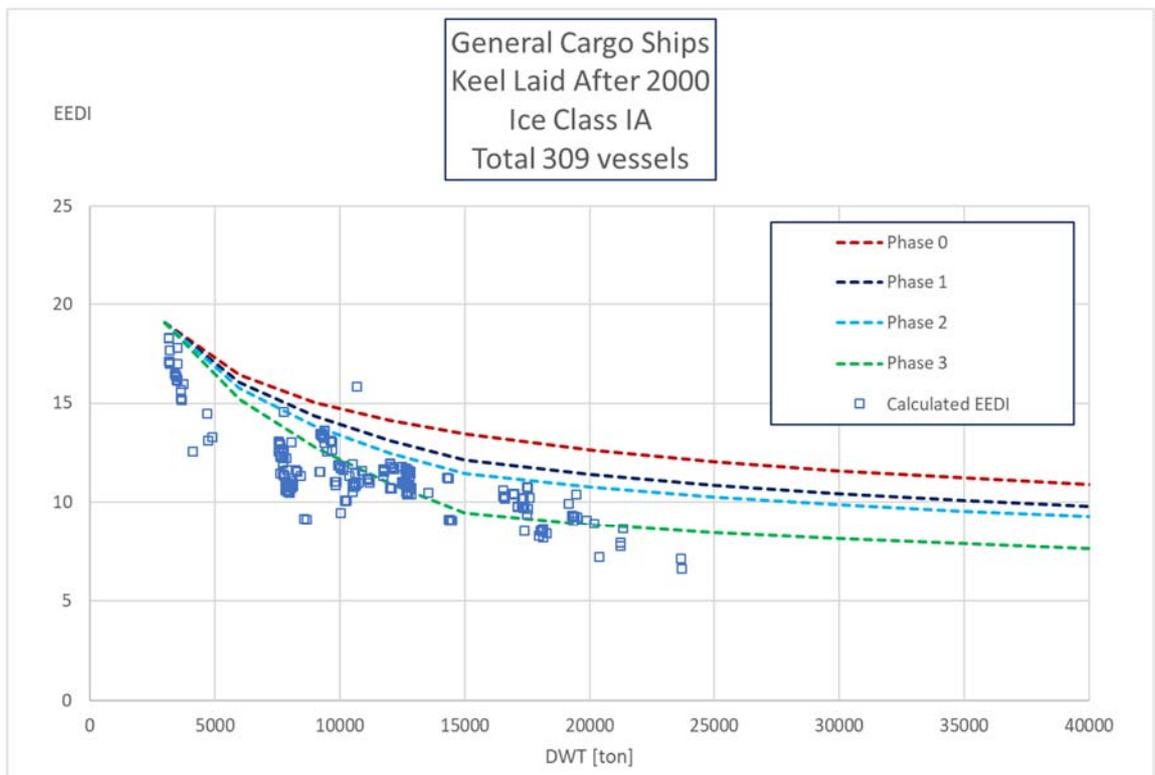
Figure 35: Calculated EEDI for general cargo ships with ice class IA with the proposed new  $f_i$  and  $f_j$ .
