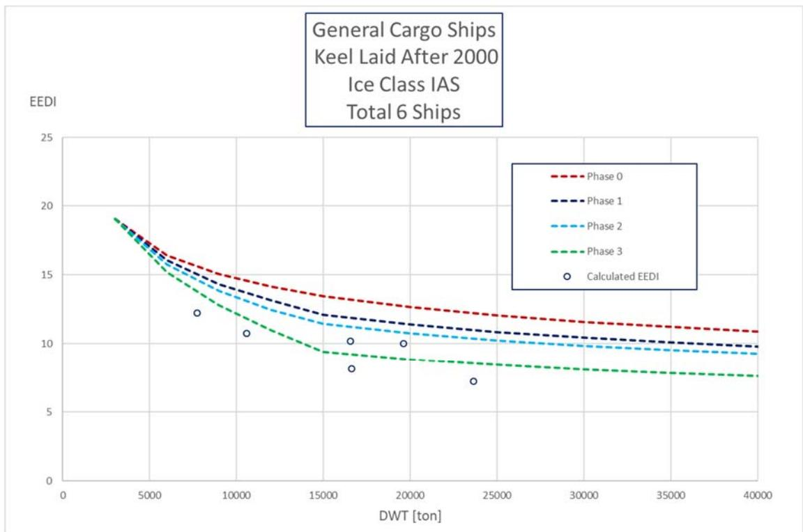
Figure 37: Calculated EEDI for general cargo ships with ice class IAS with the proposed new  $f_i$  and  $f_j$ .
