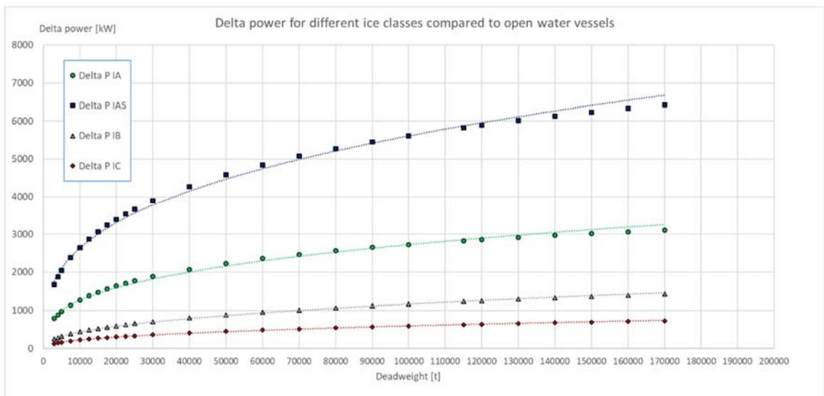
Figure 3: Difference in average engine power (MCR) of tankers having an ice class compared to open water tankers.
