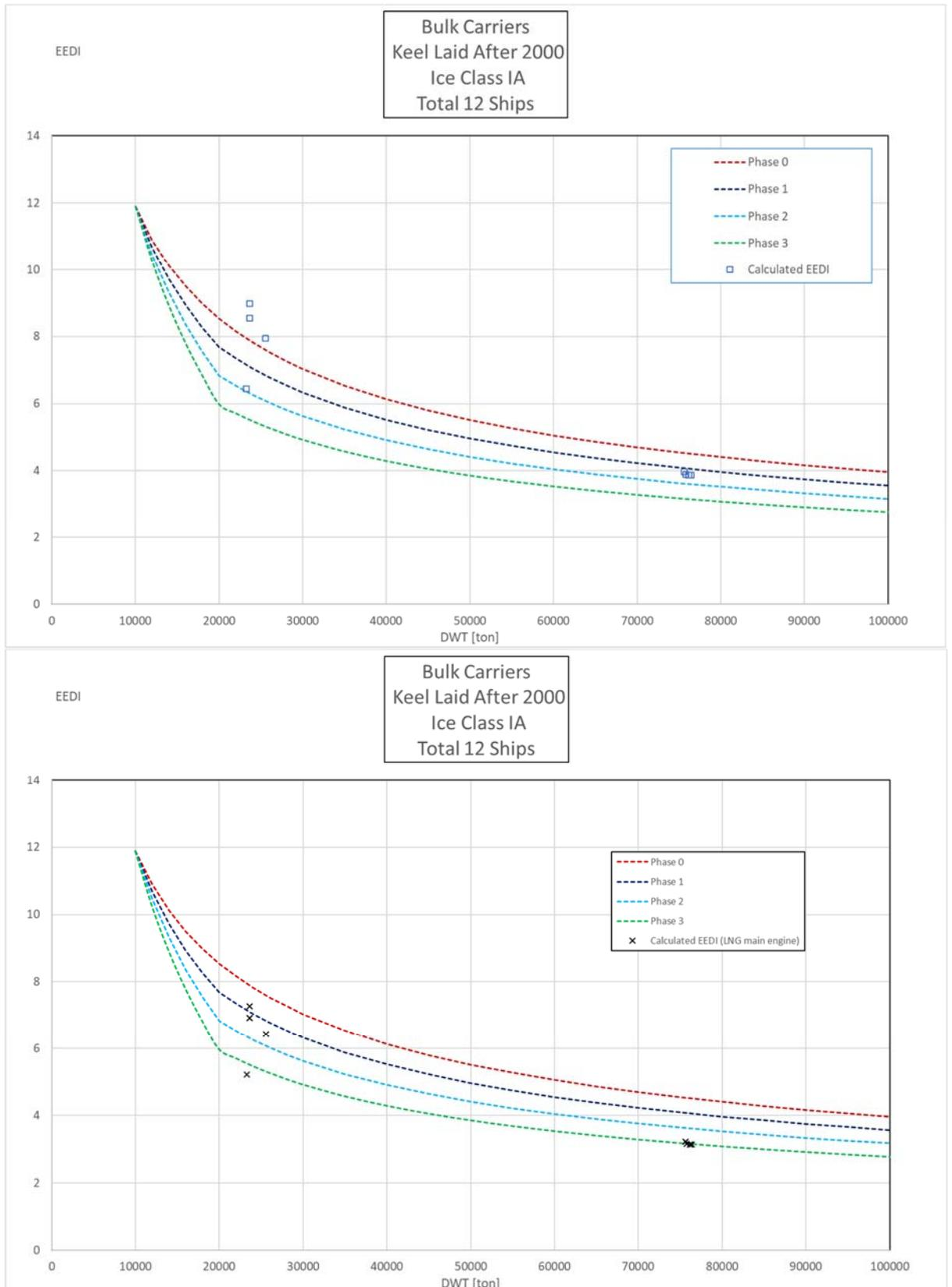
Figure 40: Comparison of calculated EEDI for MDO and LNG as fuel, bulk carriers in ice class IA.
