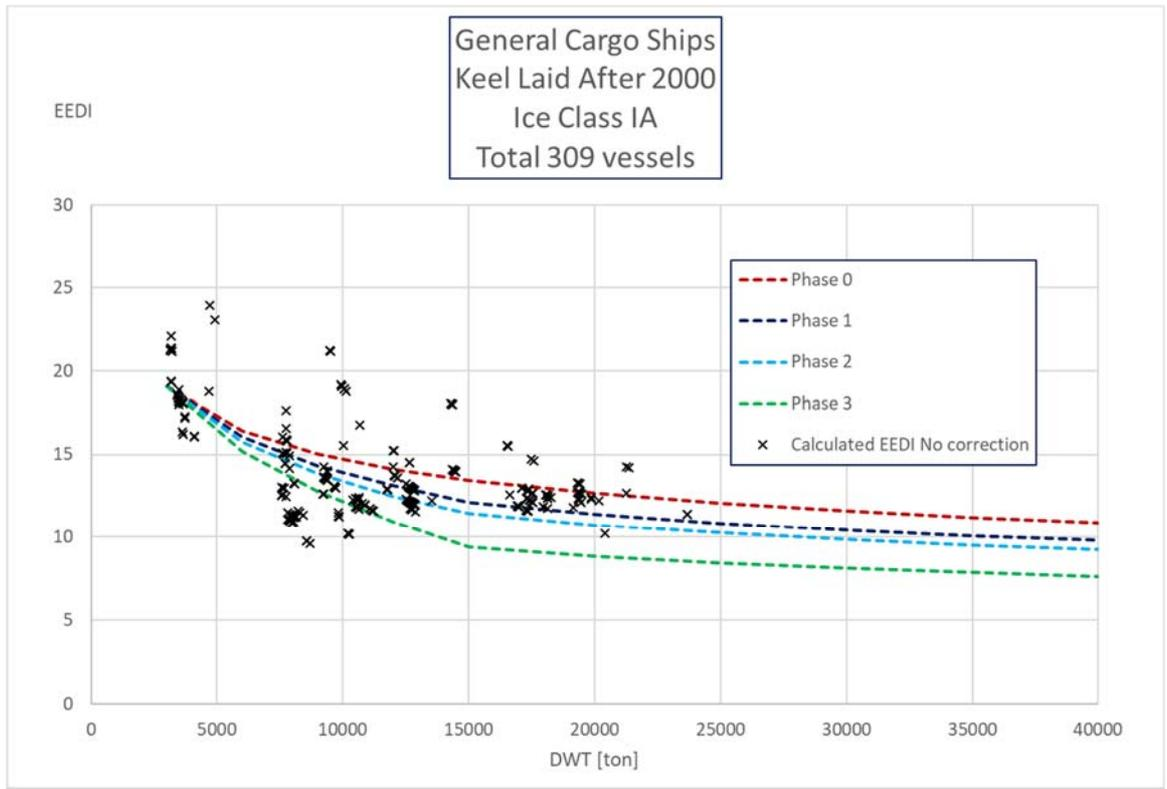
Figure 34: Calculated EEDI for general cargo ships with ice class IA without correction ( $f_i = f_j = 1$ ).
