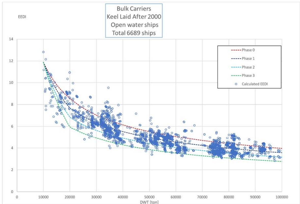
Figure 20: Calculated EEDI values for the studied open water bulk carriers.
