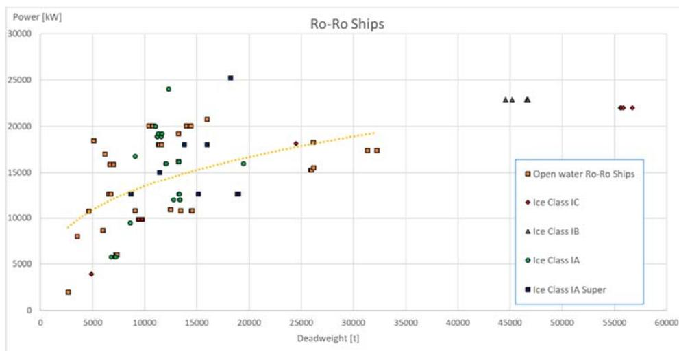
Figure 9: Average engine power of existing ro-ro ships with and without an ice class.
