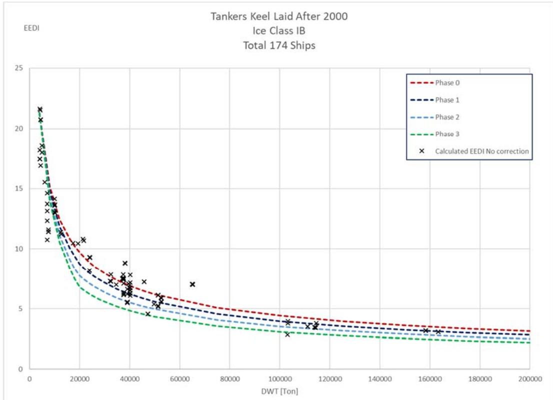
Figure 14: Calculated EEDI for tankers with ice class IB without correction ( $f_i = f_j = 1$ ).
