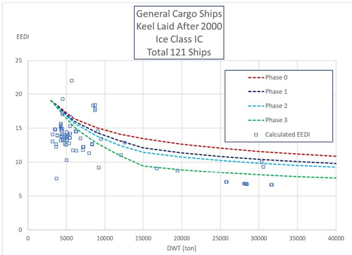
Figure 31: Calculated EEDI for general cargo ships with ice class IC with the proposed new  $f_i$  and  $f_j$ .
