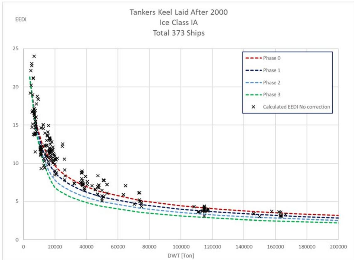
Figure 16: Calculated EEDI for tankers with ice class IA without correction ( $f_i = f_j = 1$ ).
