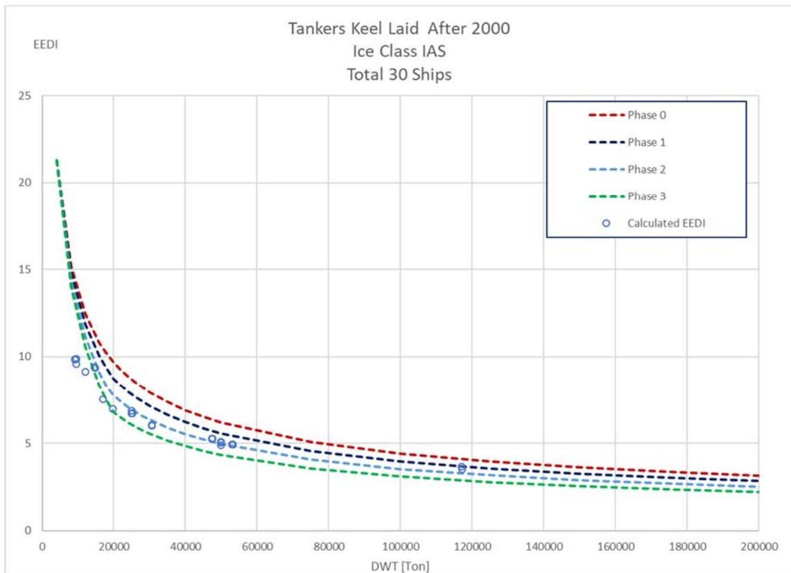
Figure 19: Calculated EEDI for tankers with ice class IAS with the proposed new  $f_i$  and  $f_j$ .
