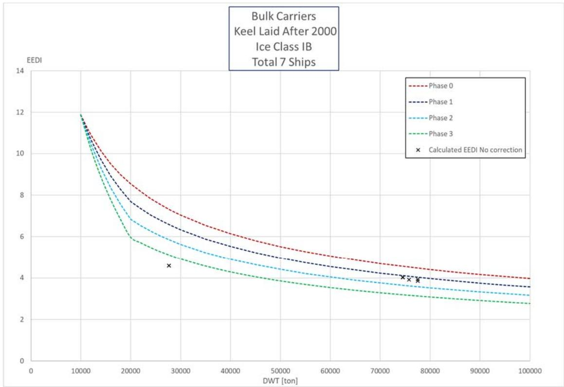
Figure 23: Calculated EEDI for bulk carriers with ice class IB without correction ( $f_i = f_j = 1$ ).
