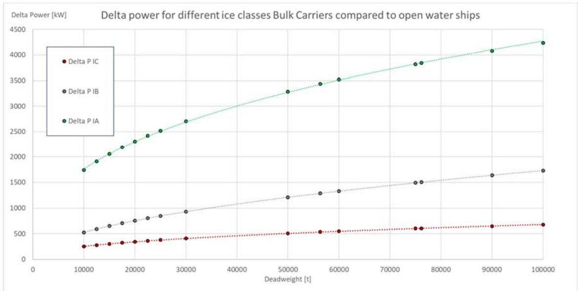
Figure 5: Difference in average engine power of bulk carriers having an ice class compared to open water bulk carriers.
