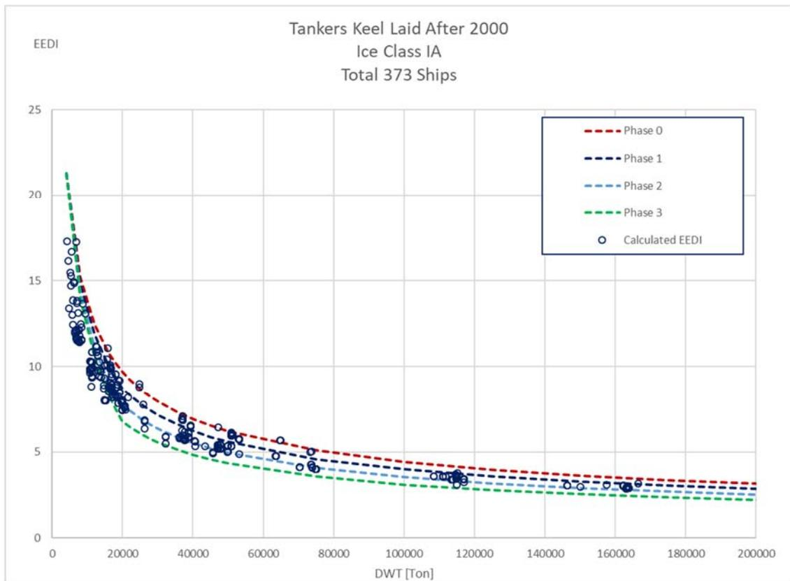
Figure 17: Calculated EEDI for tankers with ice class IA with the proposed new  $f_i$  and  $f_j$ .
