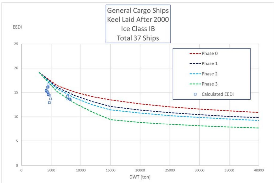
Figure 33: Calculated EEDI for general cargo ships with ice class IB with the proposed new  $f_i$  and  $f_j$ .
