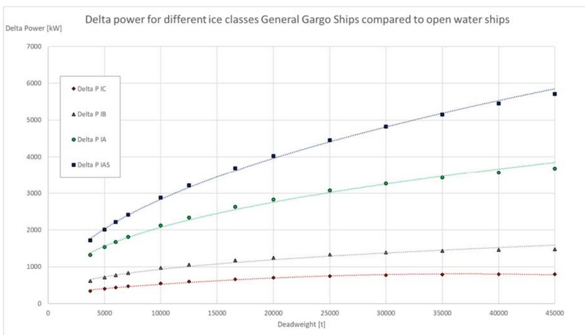
*Figure 7: Difference in engine power of general cargo ships having an ice class compared to open water general cargo ships.*
