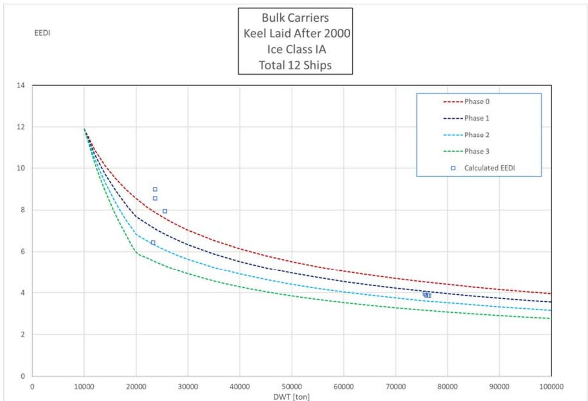
Figure 26: Calculated EEDI for bulk carriers with ice class IA with the proposed new  $f_i$  and  $f_j$ .
