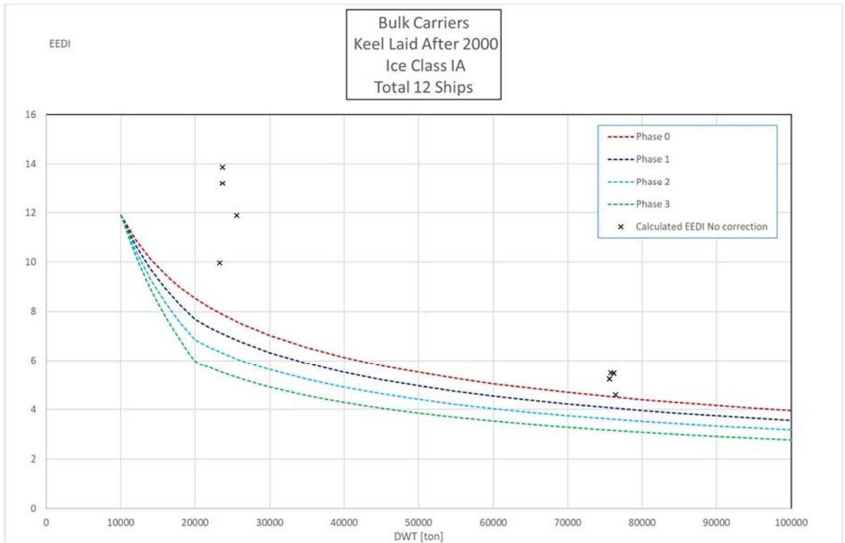
Figure 25: Calculated EEDI for bulk carriers with ice class IA without correction ( $f_i = f_j = 1$ ).
