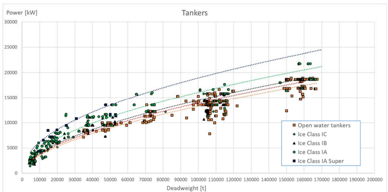
*Figure 2: Average engine power of existing tankers with and without an ice class.*
