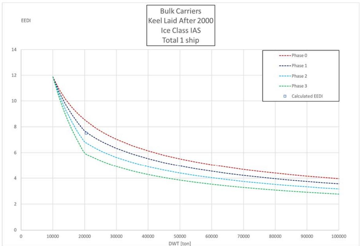
Figure 28: Calculated EEDI for bulk carriers with ice class IAS with the proposed new  $f_i$  and  $f_j$ .
