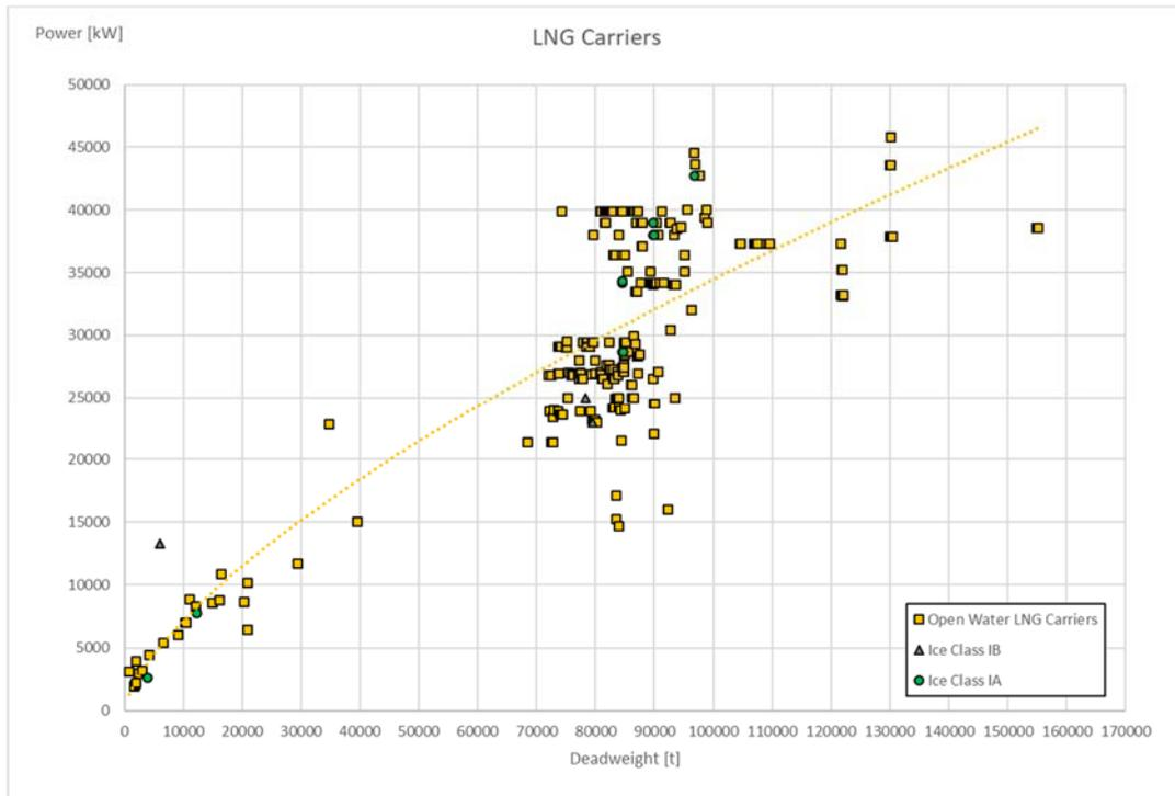
Figure 10: Average engine power of existing LNG carriers with and without an ice class.
