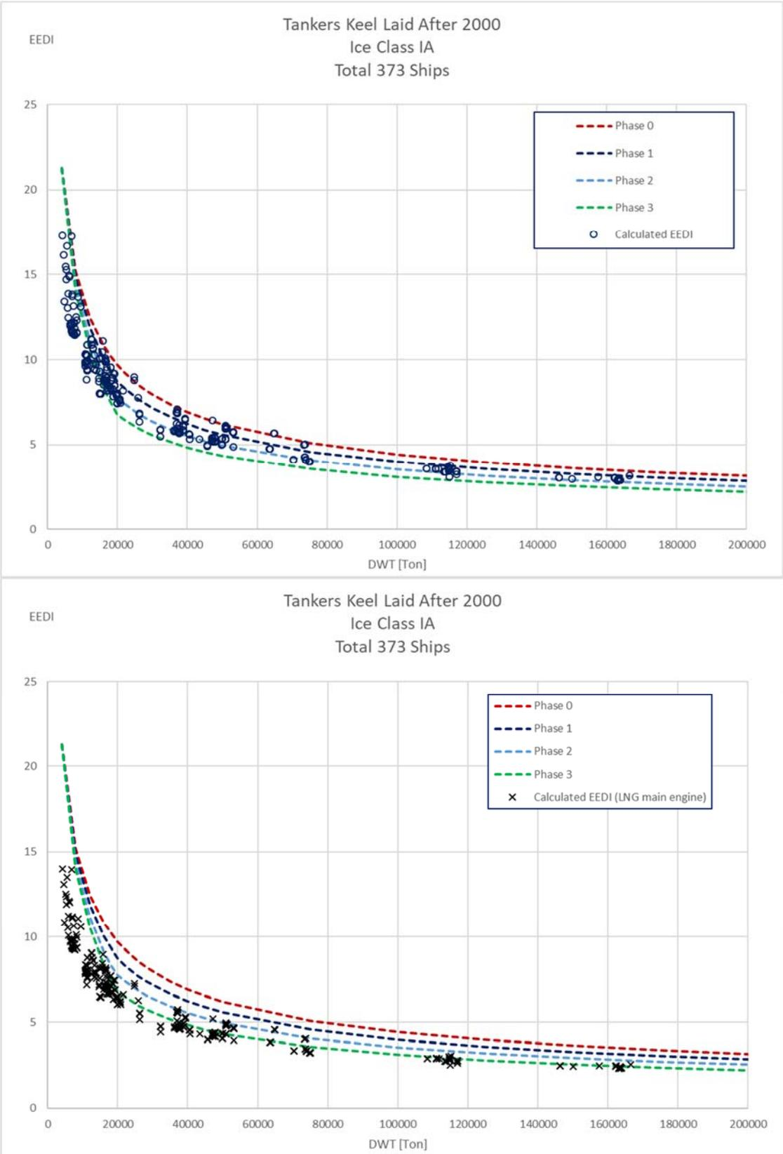
Figure 38: Comparison of calculated EEDI for MDO and LNG as fuel, tankers in ice class IA.
