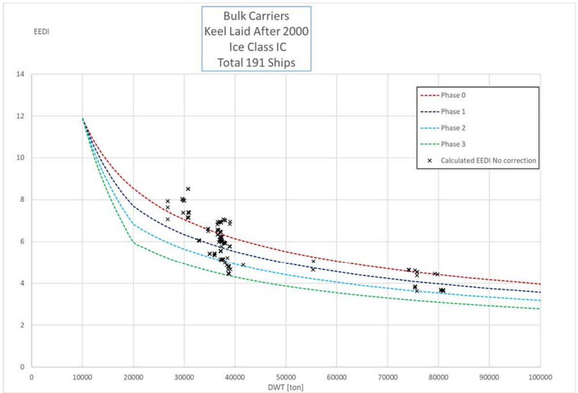
Figure 21: Calculated EEDI for bulk carriers with ice class IC without correction ( $f_i = f_j = 1$ ).
