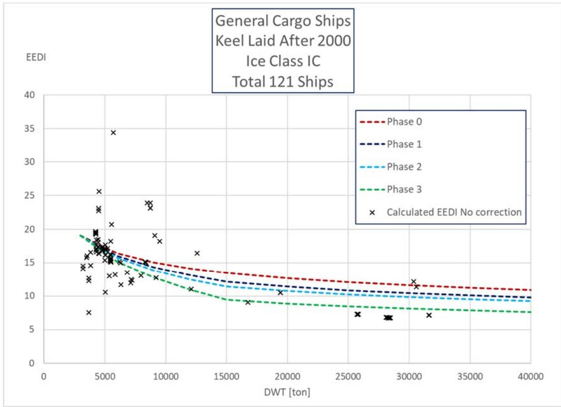
Figure 30: Calculated EEDI for general cargo ships with ice class IC without correction ( $f_i \equiv f_j = 1$ ).
