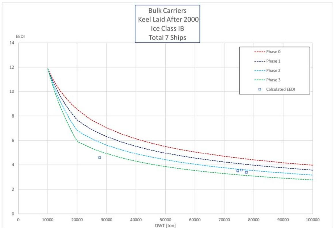
Figure 24: Calculated EEDI for bulk carriers with ice class IB with the proposed new  $f_i$  and  $f_j$ .
