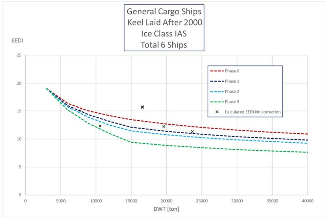
Figure 36: Calculated EEDI for general cargo ships with ice class IAS without correction ( $f_i = f_j = 1$ ).
