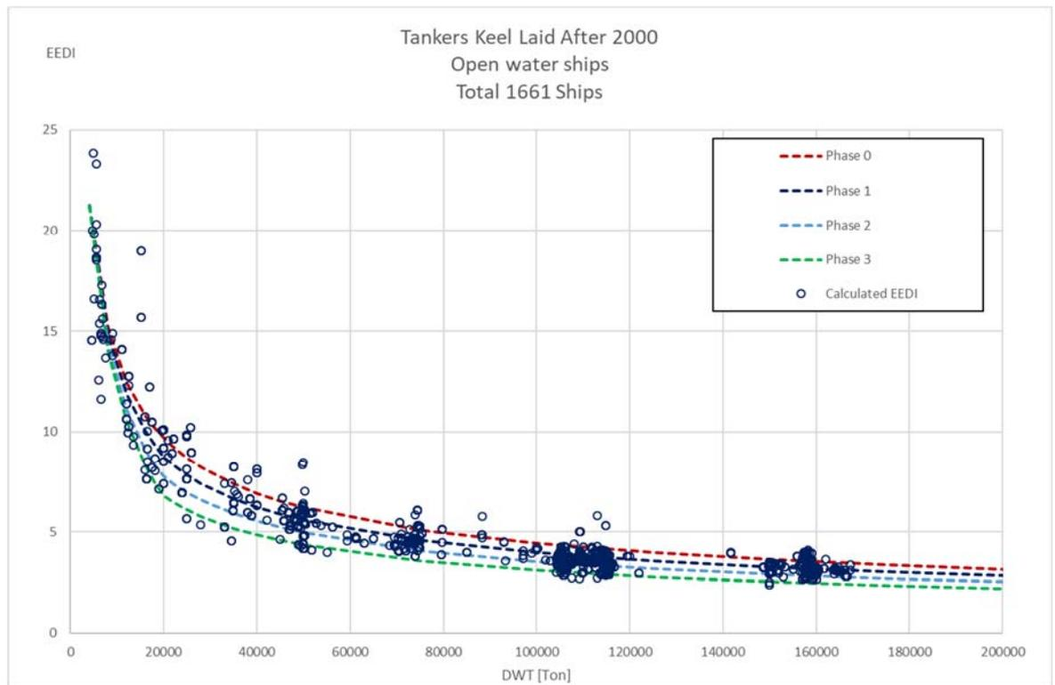
Figure 11: Calculated EEDI values for the studied open water tankers.
