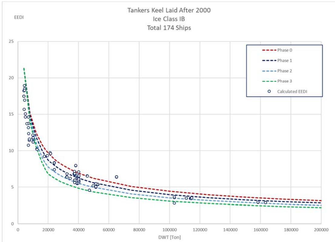
Figure 15: Calculated EEDI for tankers with ice class IB with the proposed new  $f_i$  and  $f_j$ .
