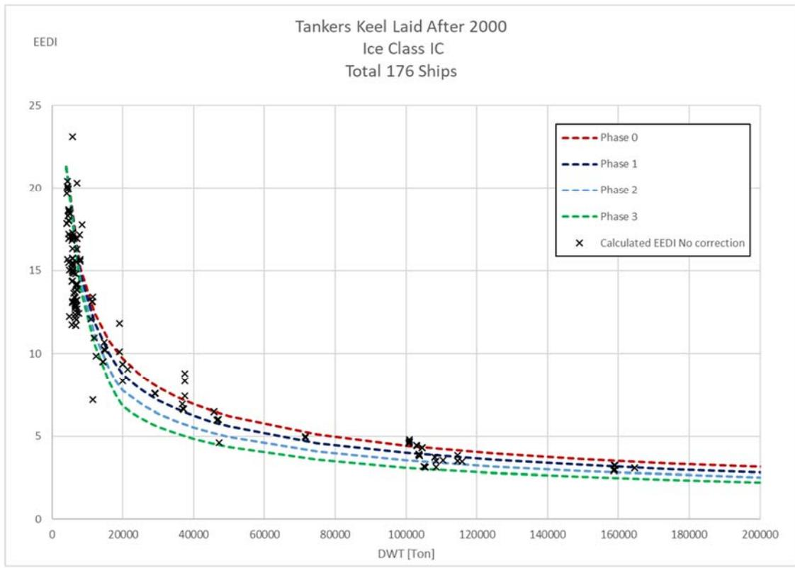
Figure 12: Calculated EEDI for tankers with ice class IC without correction ( $f_i = f_j = 1$ ).
