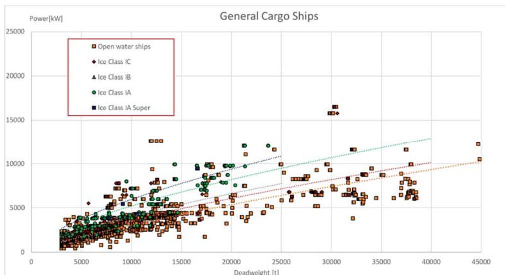
*Figure 6: Average engine power of existing general cargo ships with and without an ice class.*
