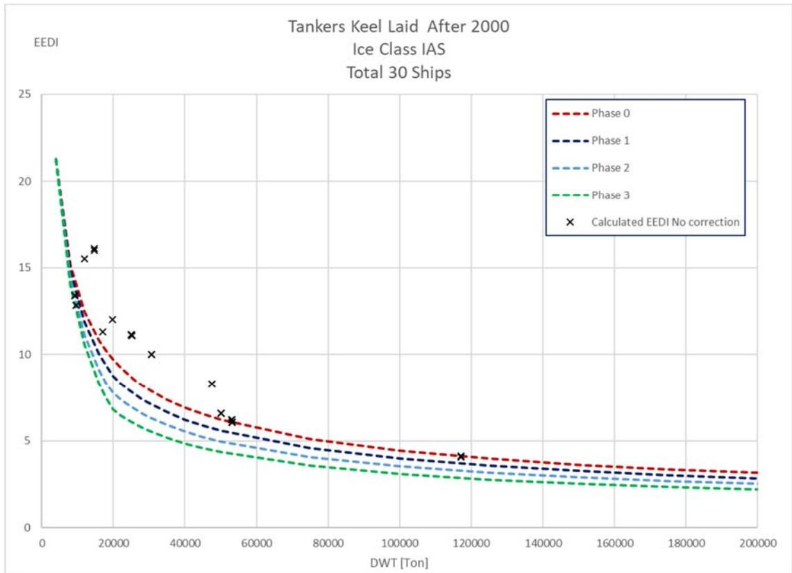
Figure 18: Calculated EEDI for tankers with ice class IAS without correction ( $f_i = f_j = 1$ ).
