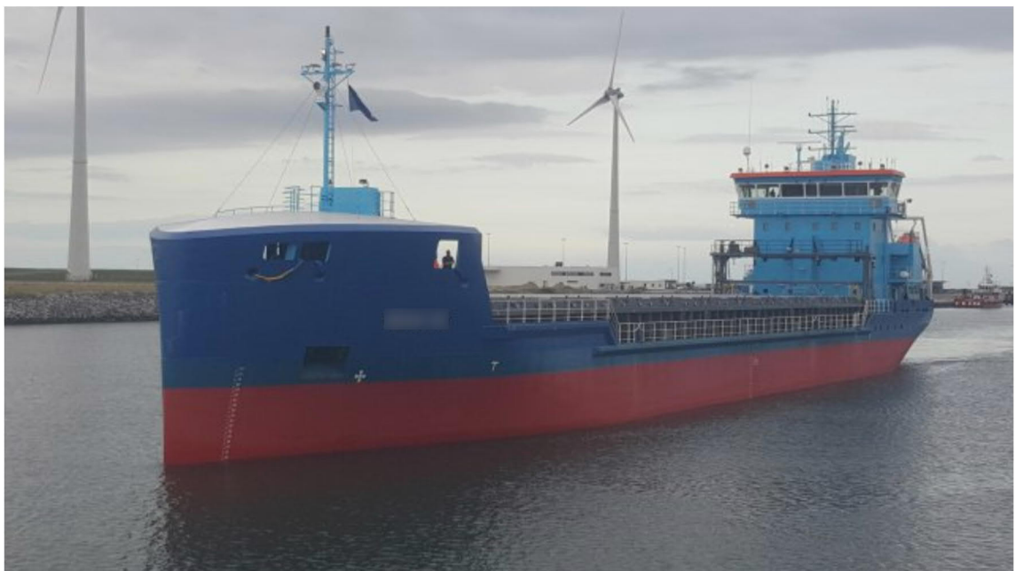
Figure 4-34: Example of an vertical bow of an EEDI compliant IA general cargo ship.
