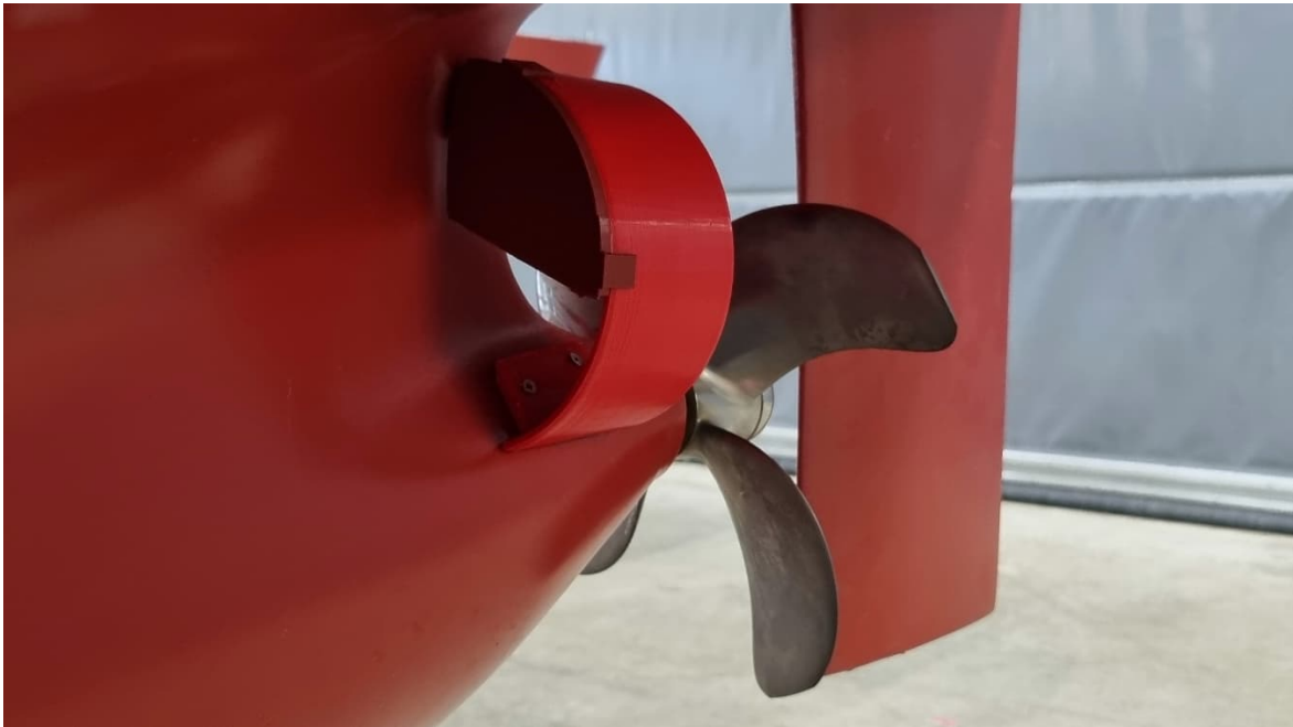
Figure 3-5: The Schneekluth -type duct 25% clogged.
