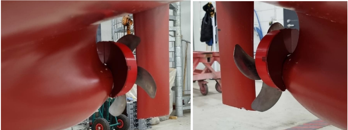
Figure 3-12: The Becker Mewis -type duct 100% clogged.
