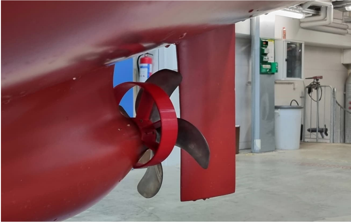
Figure 3-9: The Becker Mewis -type duct completely open without clogging.
