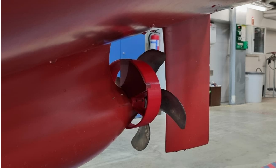
Figure 3-10: The Becker Mewis -type duct 25% clogged.
