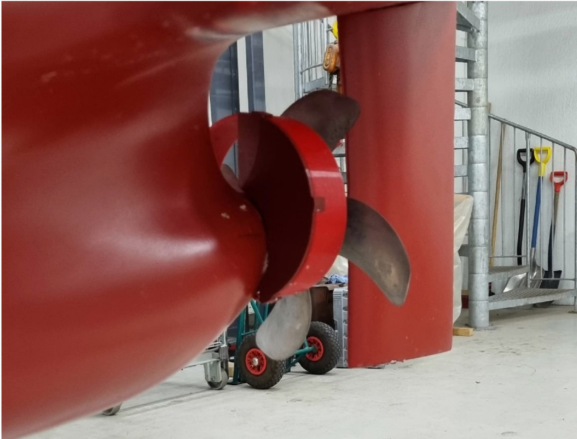
Figure 3-11: The Becker Mewis -type duct 50% clogged.
