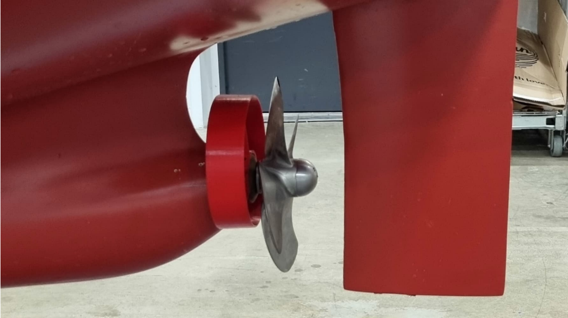
Figure 3-8: The Becker Mewis -type duct was positioned directly in front of the propeller.
