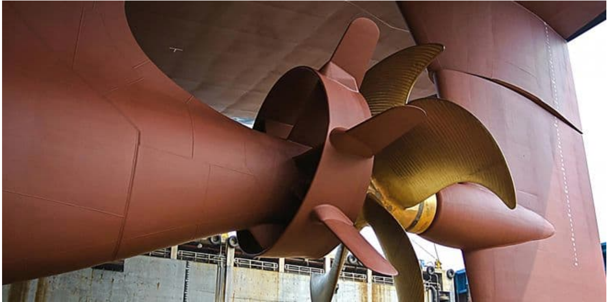
Figure 2-4: A Becker Mewis Duct with inner and outer fins. (source: https://www.becker-marine-systems.com/files/content/pdf/product_pdf/Becker_Energy-Saving_Devices.pdf )
