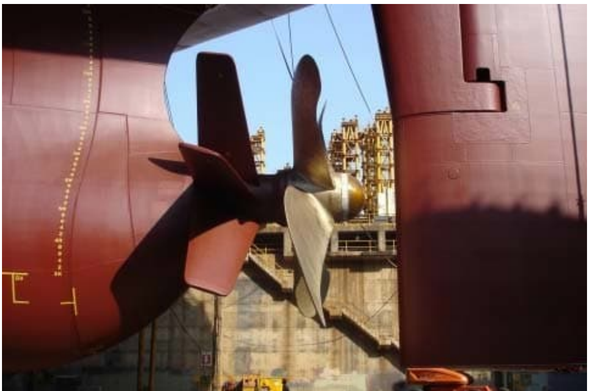
Figure 2-1: An example of PSS design, Daewoo pre-swirl stator fins [3].
